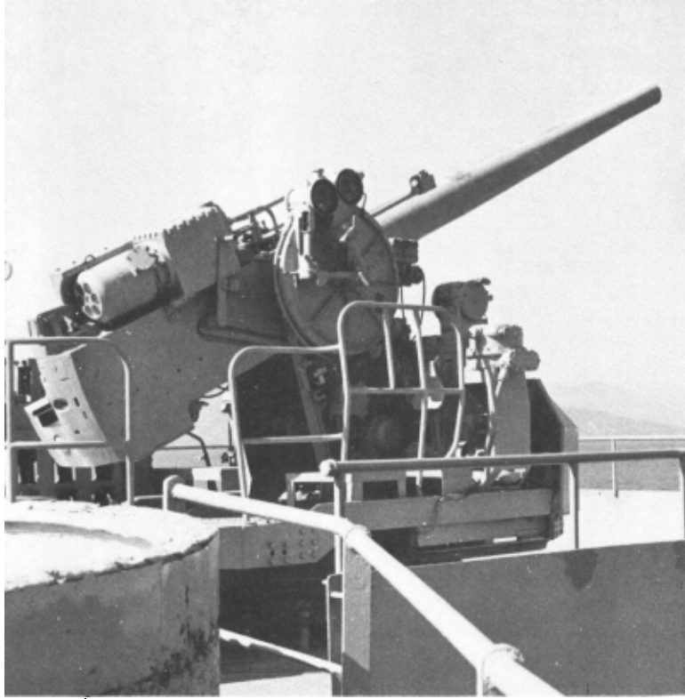
SS Jeremiah O'Brien: Stern gun tub with 5 inch/38 caliber gun. Photo: Joanie Redington
